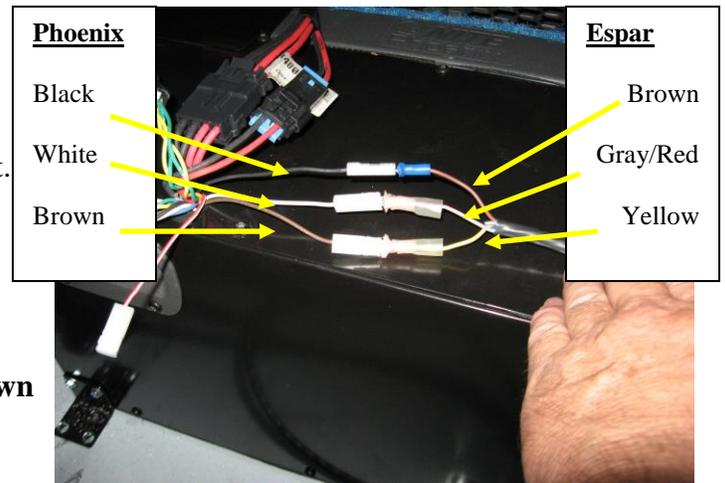
Selecting HEAT mode will turn the ENABLE signal on. The heat level will be controlled through the Phoenix (white) wire coming from the unit. This is a variable resistance signal from the Phoenix digital controller. Resistance ranges from approx. 1.8k ohms for low heat and 2.2k ohms for high heat.
