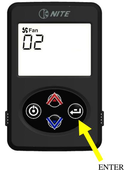
Changing TEMPERATURE set point. Anytime the temperature set point is displayed on the screen, push the up or down arrows to change. Temperature range is from 60 °F (coolest) to 85 °F (warmest).
