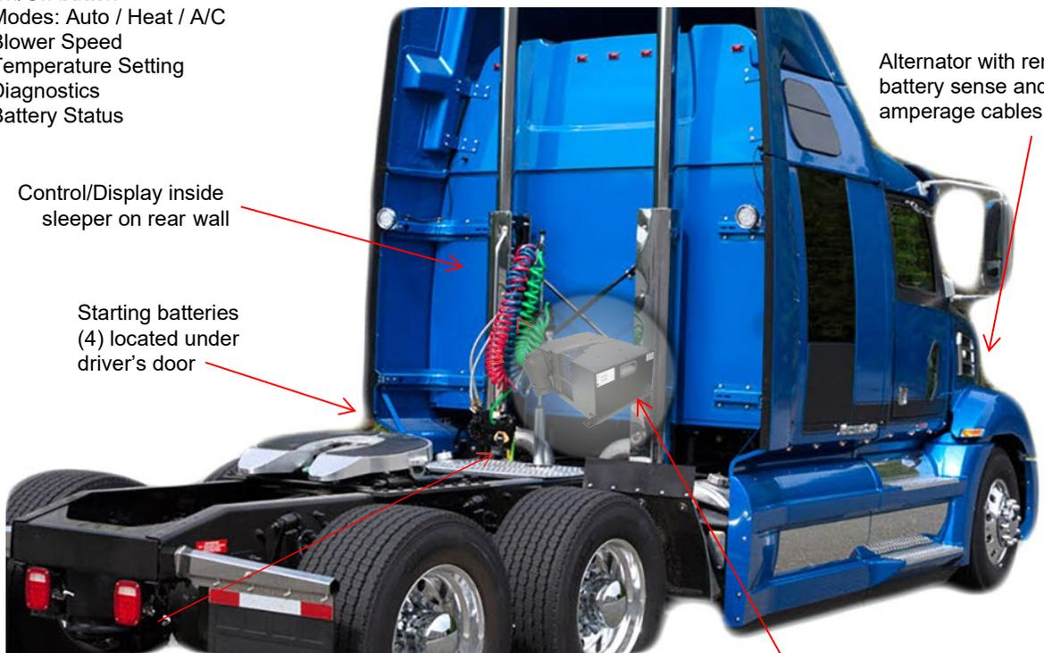
Auxiliary battery box located between the frame rails with (4) 800 CCA, AGM deep-cycle 100 Ahr minimum per batteries and Bergstrom battery management systems (BMS)
