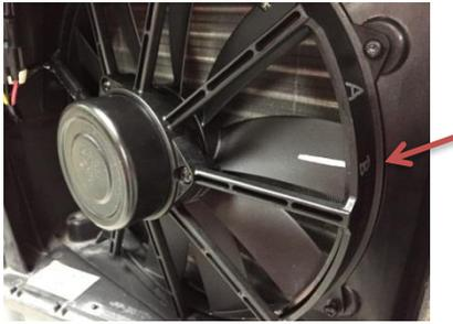
7. Rotate clockwise 1 cogging torque position and mark the third test location “C”.
