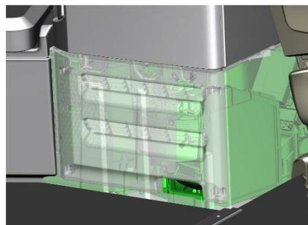
Dual HVAC System under the cabinet (evaporator, compressor, heater core, and blower)
