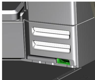
Fuel-operated hydronic coolant heater (underfloor)
