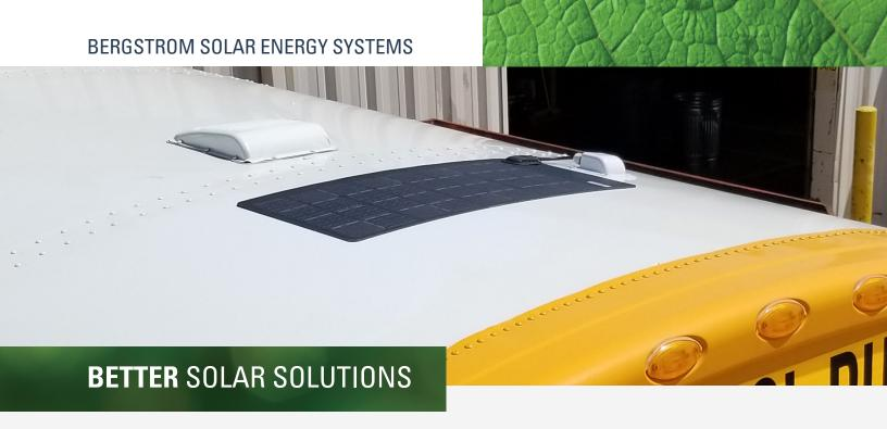
Does your bus suffer from dead batteries? Parasitic loads are on the increase and will drain the batteries when a bus sits; drastically shortening the battery life. Together with Merlin Solar's patented technology, Bergstrom has taken existing solar solutions to provide a better battery performance for buses. Our solar panel system is an inexpensive solution that helps offset the parasitic loads and helps avoid costly no starts resulting in poor service to passengers.
